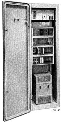
IN point to point communication systems it is necessary to site the Receiving Stations at a suitable distance from the Transmitting Stations. The Remote Control System is designed for general use with the MST range of equipments, including both transmitters and receivers. Separately sited Transmitter and Receiver Stations can be controlled from a common remote Control Centre which may be situated to suit the convenience of the system.
