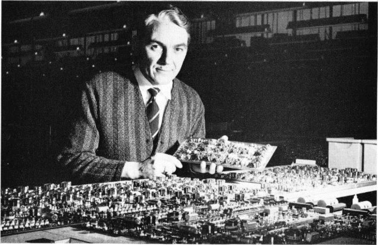
Alf Kimber, Chargehand on gantry assembly, is making spot checks on a batch of completed assemblies. He has in his hand a channel card which forms part of the multiplex equipment
