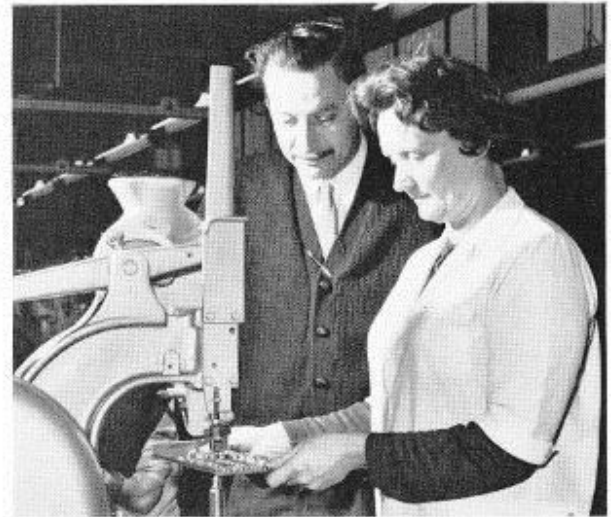
Mrs. Peggy Bibby rivets a printed board assembly to its 'package' or card-frame. With her is Laurie Langan, Chargehand on component assembly
