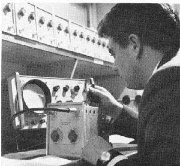
A new M.I. Attenuator, TF 2163, with a range of 0-142 dB, is in production. Chris Spooner, foreman, Attenuator Group, making a preliminary check on v.s.w.r. in the screened room. Another new attenuator is the TF 2163/M2 programmable version which is a considerable advance in remote operated attenuators
