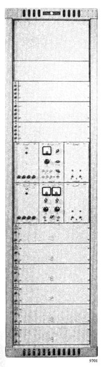
THE H 5000/H 5001 is a fully transistorized voice-frequency telegraph system for h.f radio circuits, available in a number of different versions. In the standard versions, two independent 6-channel or 12-channel transmit or receiver terminals, or one transmit and one receive terminal, are mounted in one cabinet 7 ft 6 in. high. In the transportable versions, one terminal is accommodated in a smaller size cabinet suitable for installation in a vehicle or transportable
