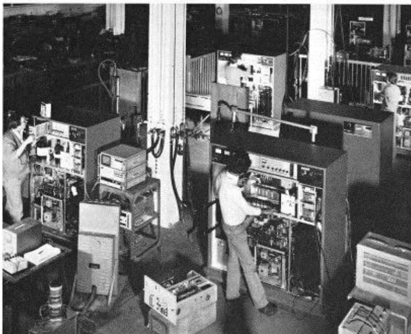
Marconi H1141 10kW amplifiers on assembly at Chelmsford
