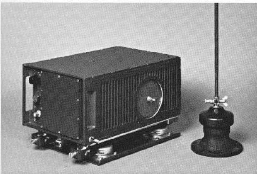
Fig. 10. 100W AMU with whip antenna
