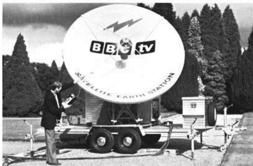
Fig. 3. Satellite earth station in use (checking stray radiation)
