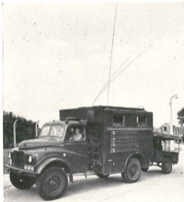
Type HS27/HR27 HF Radio Equipment installed in a vehicle.
