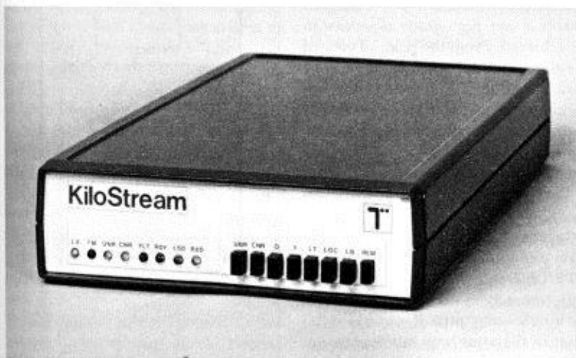
Fig. 6. Data circuit terminating equipment - DCE
