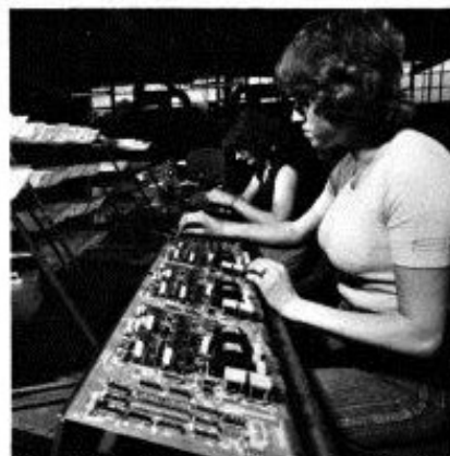
Assembling 30-channel p.c.m boards in the Chelmsford works
