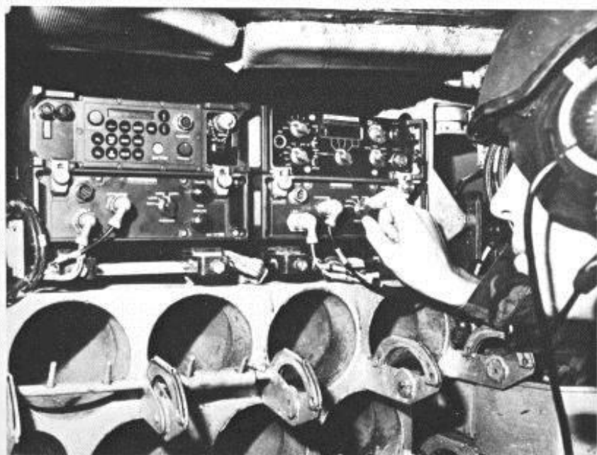
Scimitar H (left) and Scimitar V (right) each mounted in a vehicle appliqué unit fitted inside a Chieftain main battle tank
