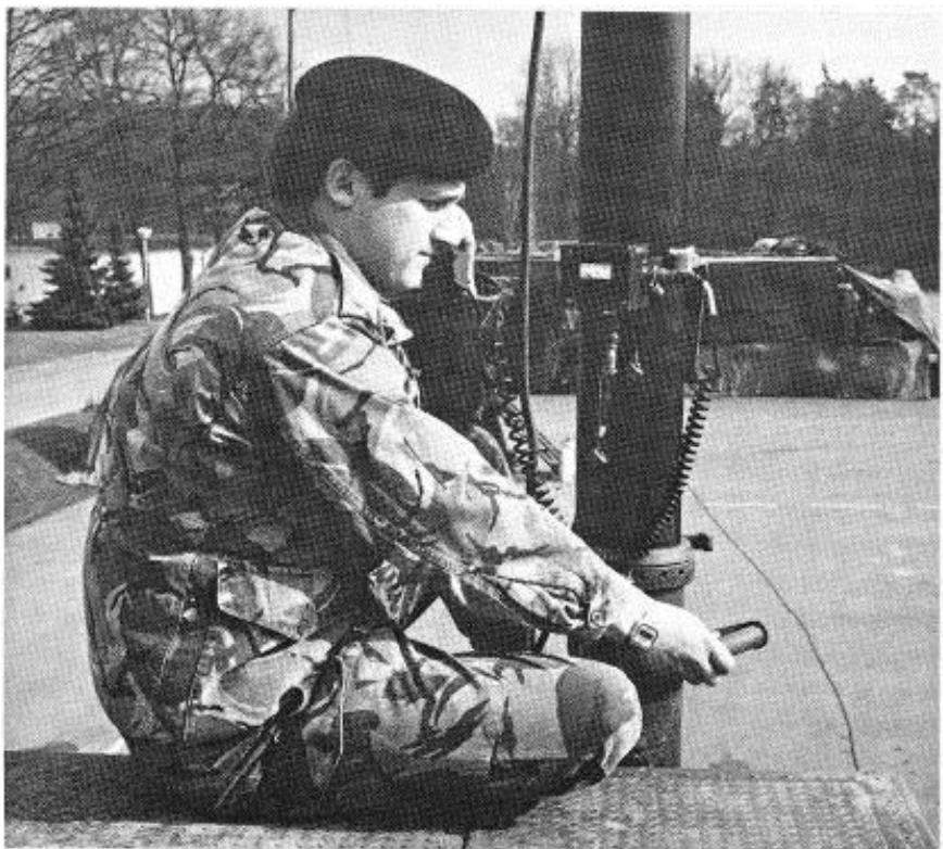
Fig. 2. The r.f meter, handset and ancillaries enable an operator simultaneously to talk to and do antenna swings with the distant station.
