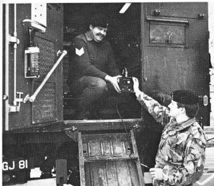
Fig. 3. The remote alarm box enables one operator to supervise more than one detachment.
