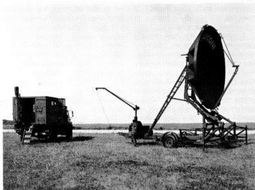
Fig. 1. Digital TACTROPO - total complement of equipment using single prime mover
