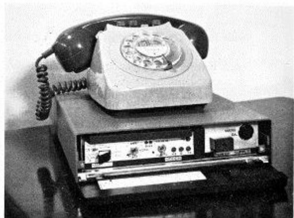
Figure 2. Modem 21 with front panel open, showing controls and power unit.
