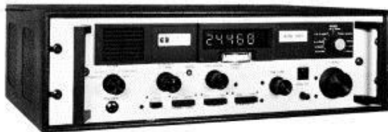
Figure 1. View of the front panel showing the LED frequency display and layout of the controls
