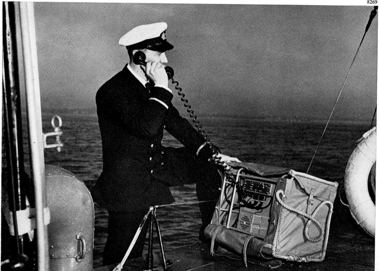
Specially made transportable VHF Radiotelephone Equipment Type HP 86B, used by Southampton Harbour Board in their aircraft control launch.
