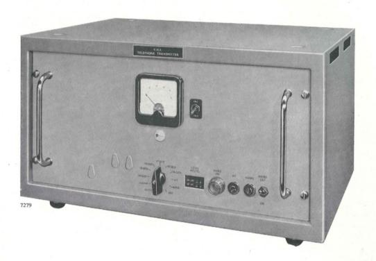
THESE TRANSMITTERS fulfil the function of headquarters transmitters working to mobile units or for point-to-point services over fixed links. Each transmitter is built on to a 19 in. panel for fitting into a bench-type cabinet or, alternatively, standard rack cabinet mounting may be employed. Their high order of frequency stability is a special feature and permits close channel operation.
