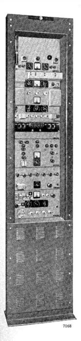
THE HM 400 SERIES TERMINALS and HM 450 Series Repeaters are UHF multi-channel equipments of the most modern design, capable of carrying one super-group, *i.e.* 60 telephone channels when associated with suitable frequency-division channelling equipment.
