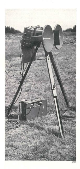
each having a 16 in. diameter spun-metal parabolic reflector. Alternatively the whole unit can be mounted in a tree or on a mast where the site is obscured. The power supply unit is normally placed on the ground in the vicinity and connected to the transmitter/receiver by a 50 ft multi-core cable. All of the equipment may be dismantled and stowed in protective cases for transportation, the heaviest single item, the power supply unit, weighing 37 lb.
