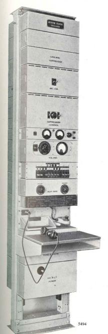
THE INTERCONNECTION of HF radio circuits with line or cable circuits presents many problems, the majority of which arise as a result of the unstable conditions on the radio portion, and it is therefore necessary to employ rather elaborate equipment if a satisfactory junction of the two transmission media is to be achieved.
