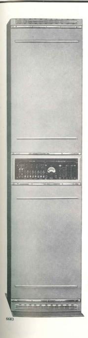
THE MARCONI-SIEMENS simplified five-band privacy equipment provides a high degree of protection against unauthorised interception of speech on a radio-telephone circuit, as compared with straightforward inversion apparatus which is intended to deal only with random interception.
