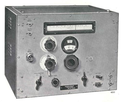
THE MEDIUM AND LONG WAVE RECEIVER Type CR200 is a self-contained receiver, designed for bench mounting and suitable for operation from AC mains, external batteries, or vibrator power-pack sources, link changeover facilities being provided.
