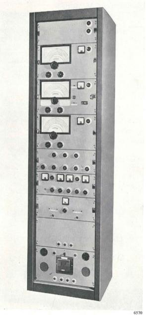
for CW on/off reception, employing intermediate frequencies of 2600 and 100 kc/s. For FSK reception a third oscillator giving an IF of 10 kc/s is also utilised.
