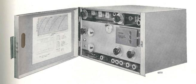
THE TYPE HR 51 RECEIVER is of the communication type, suitable for reception of telephone or telegraph signals on any one of three pre-set HF channels. The receiver may be controlled remotely over a distance of up to ten miles. The remote facilities are: control of channel selection and AF output. This control is effected over the same pair of wires that carry the audio-frequency signal output from the receiver. The control circuit must not exceed  $1000 \, \Omega$  loop resistance.
