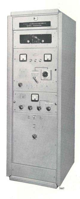
oscillator output is fed to a balanced mixer stage and mixed with the output from a four spotfrequency crystal drive oscillator. The final radiated frequency is selected by the mixer anode circuit, amplified and fed to the RF Unit. This unit contains a low-power amplifier stage coupled to the output tetrode which is matched to the aerial feeder by a  $\pi$  circuit.
