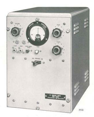
The mark condition may be set up by means of a test key and the output current is recorded on a centre-zero milliammeter.
