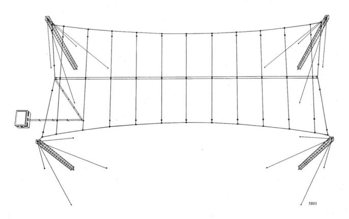
THIS IS AN OUTSTANDING ARRAY for directional reception, eminently suited for long distance point-to-point radio links. Its high forward gain and low side-lobe sensitivity result in a good signal-to-noise ratio. It gives rise to negligible reradiation and is insensitive to shadow effect.
