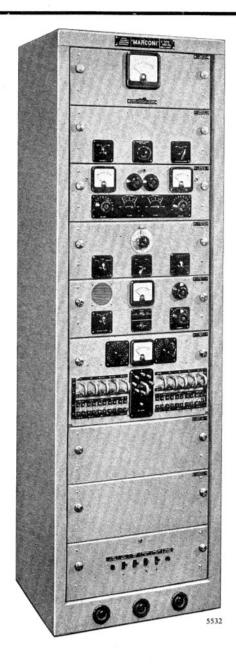
THE TYPE SSD2 EQUIPMENT supplies low-power excitation at 3·1 Mc/s, which, via an intermediate modulator, drives an HF transmitter giving the desired frequency and power output for radiating SSB telephony transmission on two independent sidebands.
