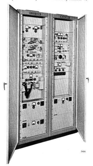
telegraph channelling equipment to give either 18 or 24 telegraph channels.
