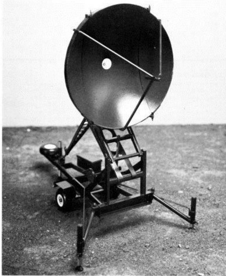
A Marconi transportable tropo antenna design
