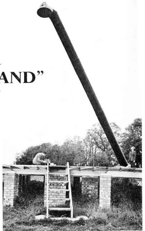
ABOVE: The aerial testing equipment at Baddow Research. J. J. Thwaites and J. H. Gibson of Aerial Section are preparing to record the directional capabilities of a model aerial
