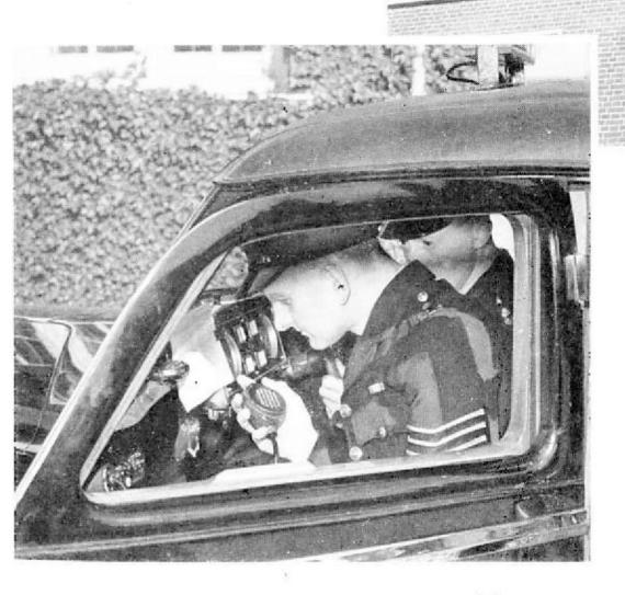
The sergeant speaks into the microphone of the control unit with built-in loudspeaker, which is fitted into the car dashboard. This Marconi unit operates the 10 watt transmitter and receiver units which are in the "boot" of the car. Within a matter of seconds the car is on its way to deal with the call
