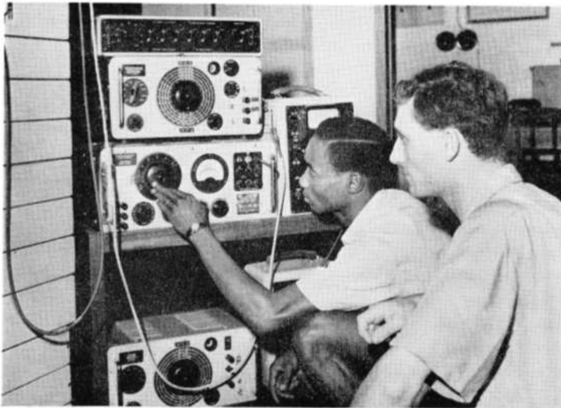
Technician under instruction while carrying out tests on channel baysides
