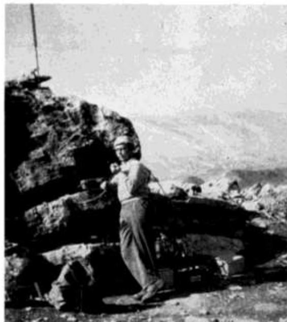
At Tang-i-Fanni Roger Gale talks on the R.T. during tests with a possible repeater site. Local people from this wild region were engaged to help carry the heavy gear to test positions
